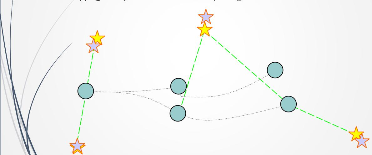
**SLAM example:** Estimate the robot's poses and the landmarks at the same time
