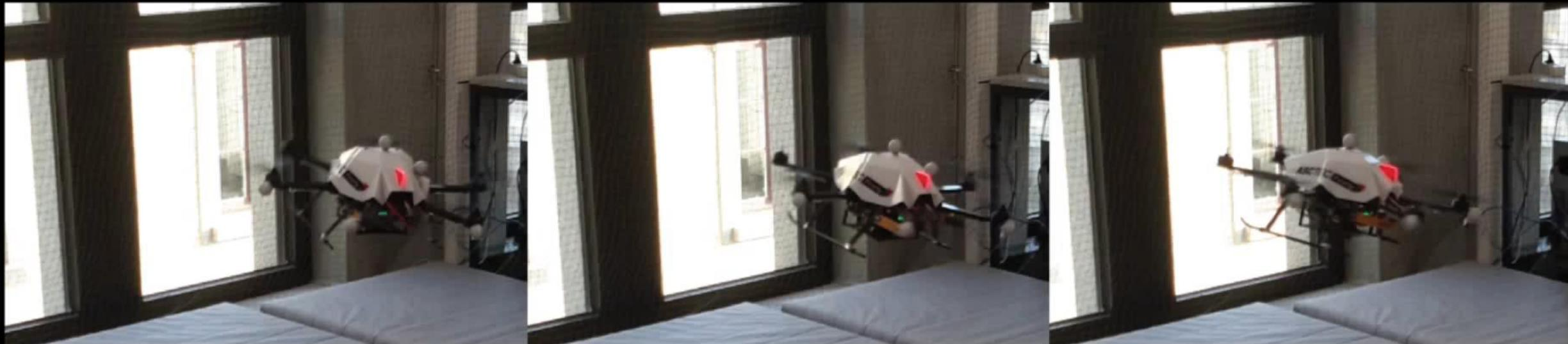
Position tracking without one propeller
