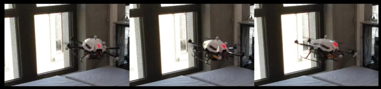
Position tracking without one propeller
