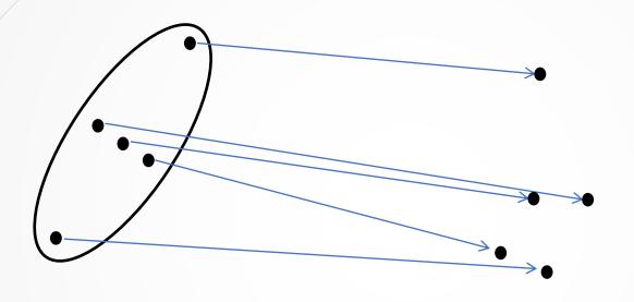
Transforms each sigma point through the non-linear function.
