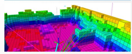
Tree-based exploration: At every iteration, nbvplanner spans a random tree of finite depth. Each vertex of the tree is annotated regarding the collected Information Gain – a metric of how much new space is going to be explored.
