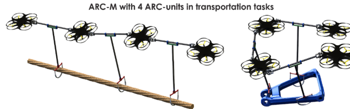
Figure 6: ARC-M system visualization with 4 ARC-units in the context of transportation tasks. Such systems can benefit from the advanced payload capabilities and the ability to morph their shape. Such a task can be achieved with a team of non-connected micro aerial vehicles but the benefit in such a case relates to the overall sensorial, processing, co-localization and control benefits of the connected system.
