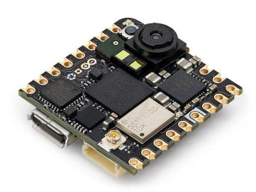
this project you are asked to develop a miniaturized visual-inertial system that exploits an integrated system that offers a monocular camera, an Inertial Measurement Unit, a 1D distance sensor (time-of-flight), alongside a processing solution integrating 1x Arm® Cortex® M7 @ 480 MHz and 1x Arm® Cortex® M4 core @ 240 MHz. Your solution should fit well in the M7 core of this system and perform visual-inertial odometry at 20FPS.
